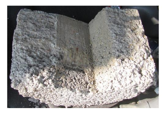
The plate tooth bending, withdrawal, and slippage of the wood was revealed after the tests by impact splitting of the concrete mass to remove it from the post.
