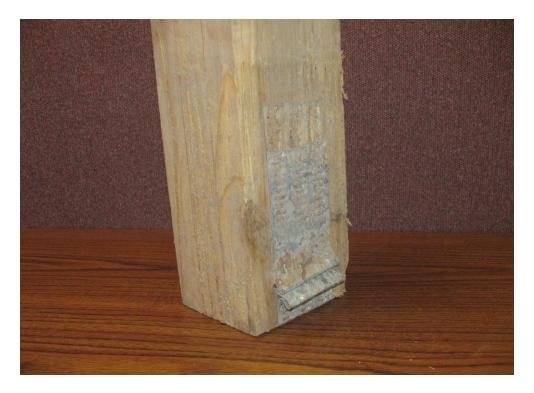
The observed mode of failure for the metal-plate-connected wood-to-concrete joint with is tooth withdrawal.
